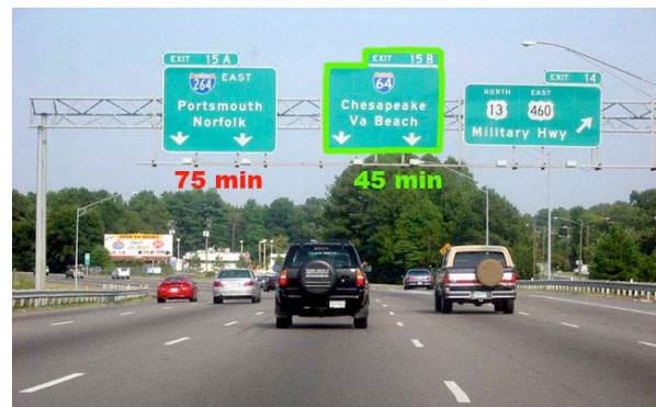
Fig. 2. An A-HUD mockup. A driver is looking straight ahead and seeing navigation directions based on traffic.
